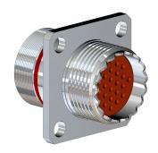
The HiRel **H2DA2\*-222** High Density Square Flange Receptacle is designed with a double start ACME thread and a threaded rear accessory. It has four holes that can be mounted and bolted to a panel and is able to accomodate a rear backshell. This H2D receptacle is available in shell sizes 5-21 with any of our standard insert arrangements as well as custom configurations.
